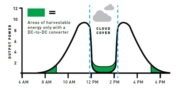
PV inverters harvest DC input when the array or string voltage is above a certain threshold. *This impacts generation at beginning of day, end of day and in heavy cloud cover.*
